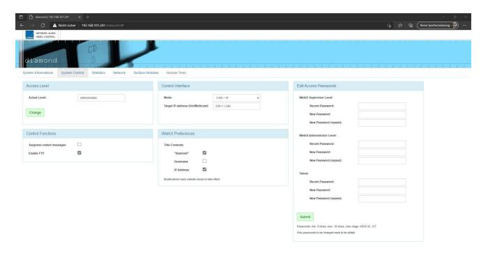
In the tab ""System Control" the communication can be established via Unicast or Multicast. The setting needs to match the according setting in the Power Core.
