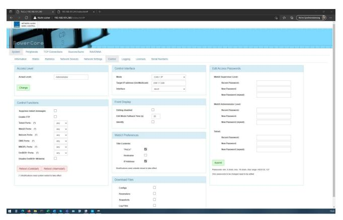
In the tabs "System" and "Control", the communication can be established via Unicast or Multicast. The setting needs to match with the according setting in the Power Core.
