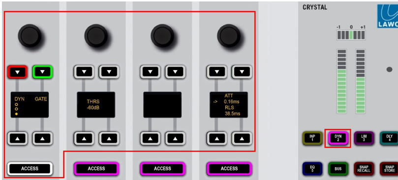
Surface Controls (Gate)
