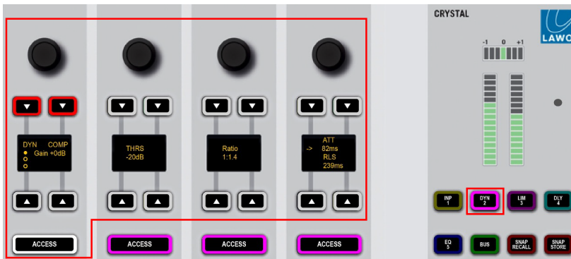
Surface Controls (Compressor)
