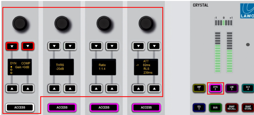
Surface Controls (Compressor)
