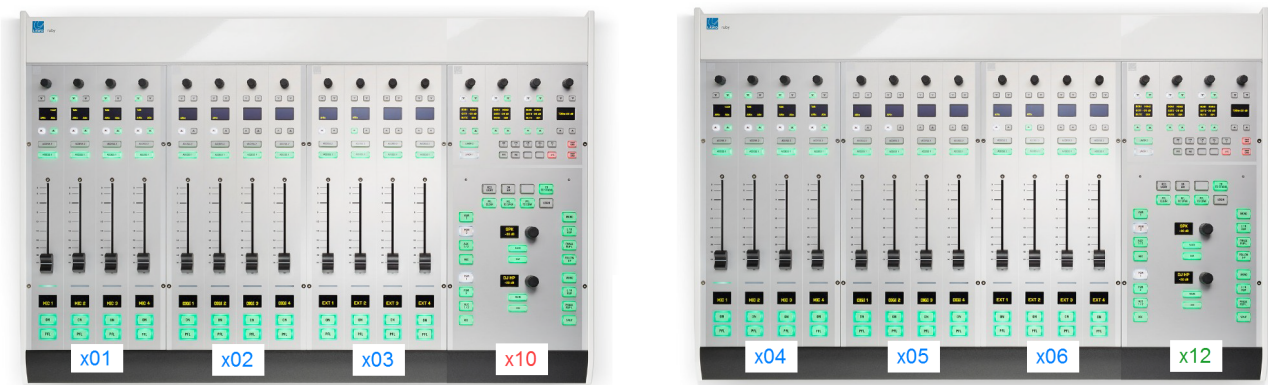
Console: CAN Bus Addresses (hexadecimal)
