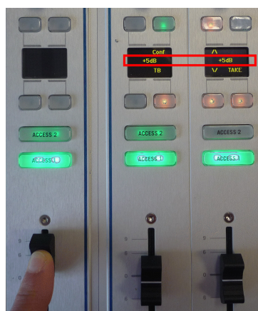
Combined level shown in slave fader displays
