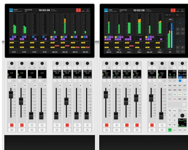
The number of channel strips and master slots should match the controls on the surface modules. For crystal, there are two possible layouts: a Fader session (with 8 channel strips) or a Main session (with 6 channel strips plus 2 master slots).
