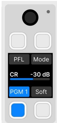
For the Control Room (CR) output, the rotary control adjusts a single parameter: monitor level. The display shows the control's function and current value. The current monitor source is highlighted in blue (e.g. PGM 1).
