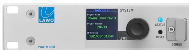
If the **STATUS** LED does not start to blink, then the device has an internal problem. Please reboot the device (using the **RESET** button) as a first step.
